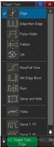
Figure 41. Wide array of advanced parametric trigger modes.
