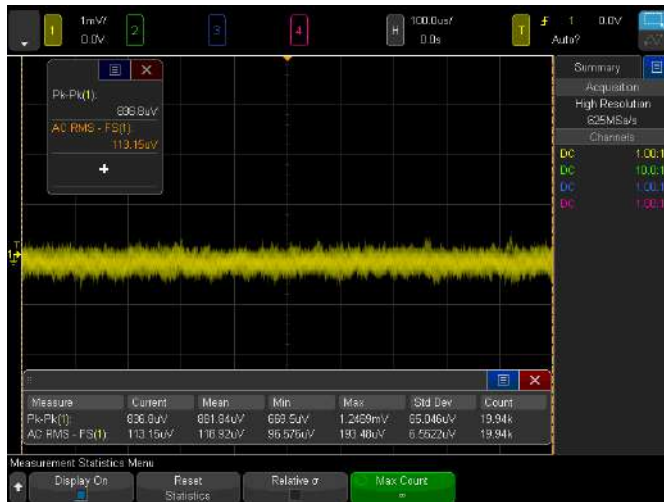
Figure 40. Getting 113 \mu\text{Vrms} noise floor at 1 mV/div with the high-resolution mode.
