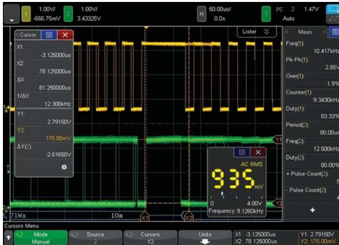
Figure 13. See 10 measurements, cursor information, and the DVM simultaneously by dragging the desired docking panel to any open area.
