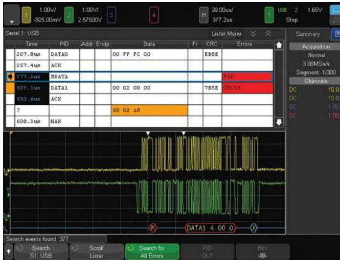
Figure 21. USB 2.0 trigger, decode and "lister" display.
