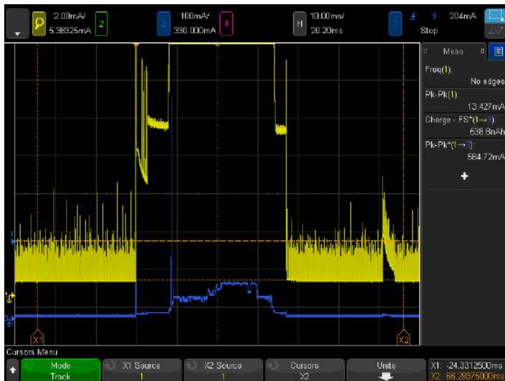
Figure 35. The 4000 X-Series and N2820A Series high-sensitivity current probe measuring > 500 mA and < 1 mA current simultaneously.
