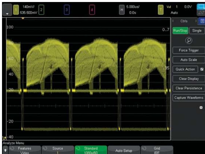
Figure 27. Triggering on 1080p HDTV signal analysis.
