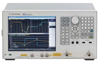
Figure 4b. The Agilent E5061B ENA Series Network Analyzer measures S-parameters
