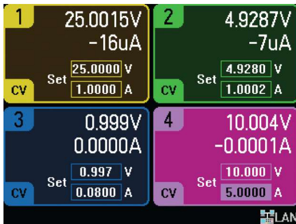
Figure 2. In Meter View, all 4 outputs can be viewed simultaneously. The both measured values for voltage and current and setting for voltage and current are displayed for each output.
