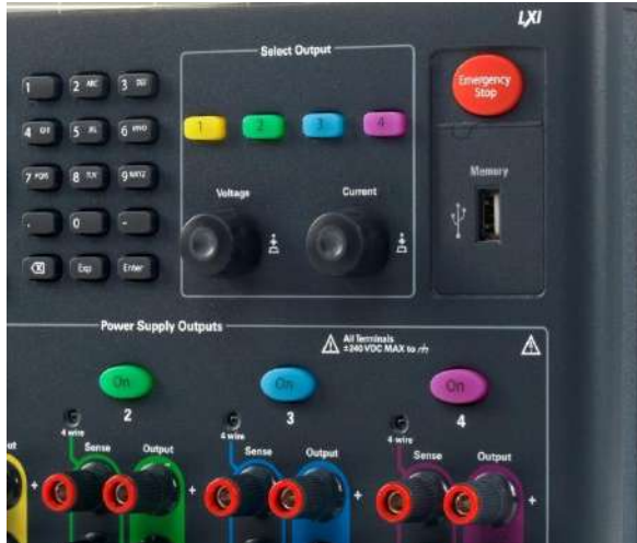
Figure 11. The N6705's front panel USB port.
