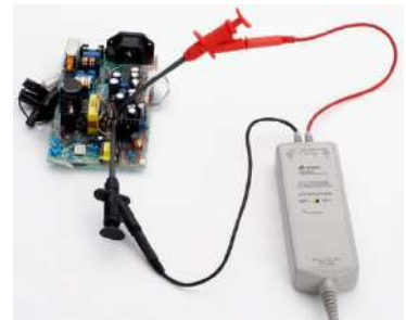
N2790A measuring a power supply signal
