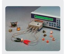
The 4263B LCR meter is a costeffective universal LCR meter, designed for both production tests and evaluating a variety of components.
