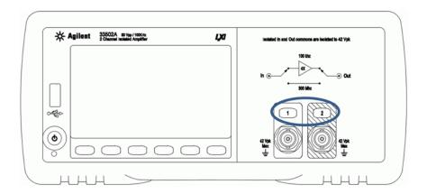
When you turn a channel on, the number on the button illuminates, as shown below for channel 1.
