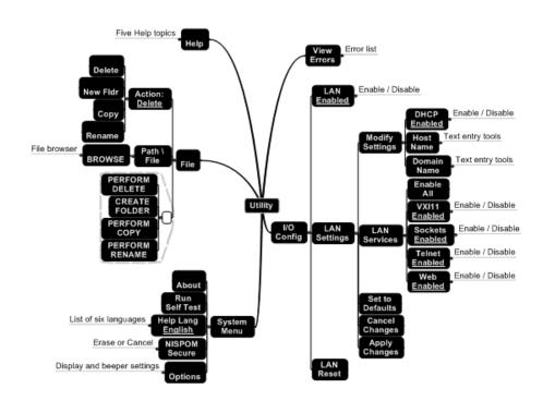
View Errors Allows you to view the instrument's error queue. Errors are cleared from the queue as they are displayed on the screen.
